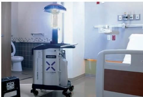
**Striking solution** // LightStrike robots use pulsed xenon (not mercury bulbs) to create full-spectrum germicidal light that quickly destroys pathogens that can cause infections. **Xenex Disinfection Services**
